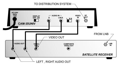
**Note:** If mono receiver is used, audio may be connected to either audio jack on **CAM-35UNIV**
